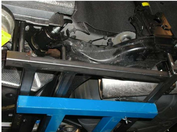
Correct installation of the rear suspension axle requires the tool 200004400 to ensure axle is accurately centred with the bodyshell; the tool has four pins on each side; one pin connects to the axle and the other one provides correct location to the bodyshell; another pin helps support the axle, and the fourth pin connects to the bush plate.
