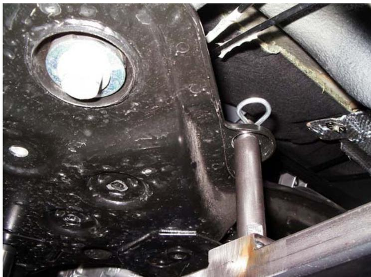
One of the crossbeam pins has a split pin to ensure safety on disassembly
