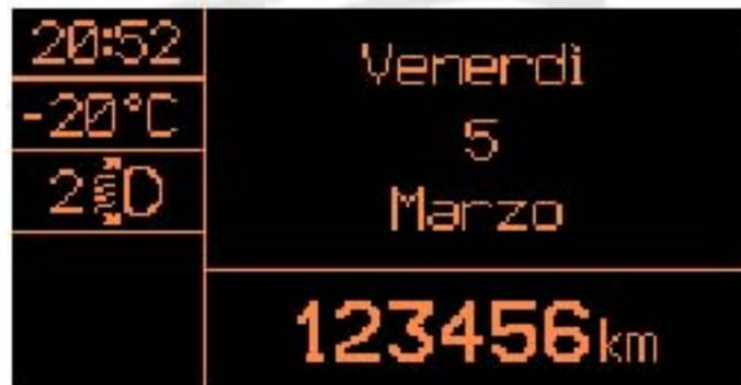
The MATRIX Dashboard adopted for the Blue&Me C3 option and Sport trim levels incorporates a reconfigurable matrix display connected to the CAN network; it comes in a standard version for both left and right drive and includes:
