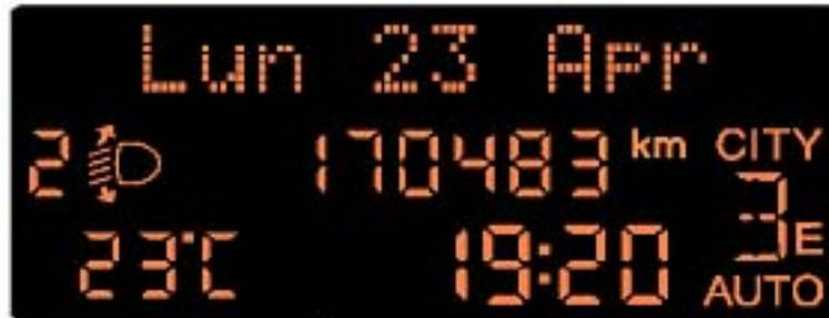
The COMFORT Dashboard adopted for the basic trim levels incorporates an alphanumeric display connected to the CAN network; it comes in a standard version for both left and right drive and includes:
