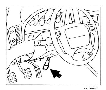
Connect the diagnostic equipment to the socket inside the vehicle.
