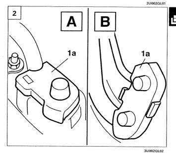
2. Open the plastic protection (1a) for the alternator electrical connections.
