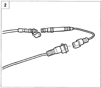
2. Wire the pressure transducer as illustrated in the diagram.
