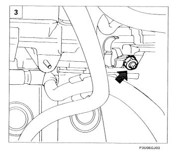
3. Undo the remaining fixing nut illustrated in the diagram and carefully remove the distribution manifold.
