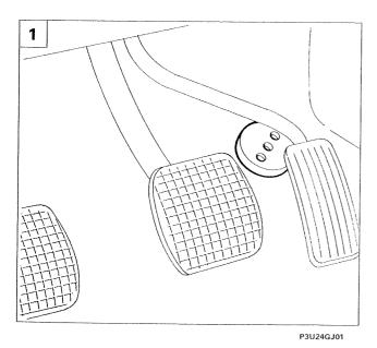
1. To correct the voltage values with the accelerator in the maximum position, requlate the adjustment device and repeat the procedure using the diagnostic equipment.
