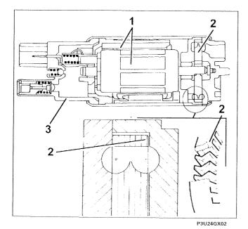
The electric fuel pump has a permanent magnet electric motor (1) which drives the pump (2) impeller and a support cover (3) which contains the electrical and hydraulic connections
