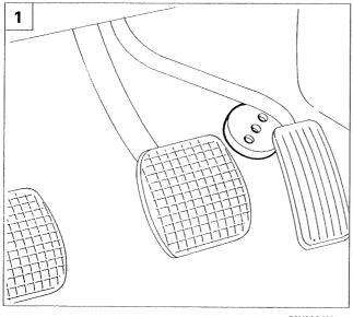
celerator in the maximum position, regulate the adjustment device and repeat the procedure using the diagnostic equipment.
