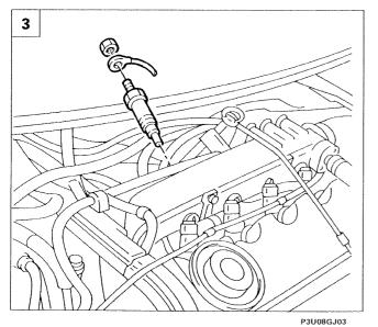
3. Disconnect the electrical connection, undo the fixing nut and remove the heater plugs using a suitable spanner.
