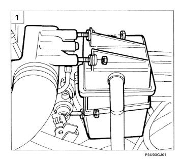
1. Move the oil vapour separator aside undoing the three fixing nuts.
