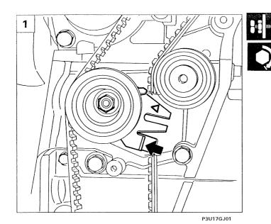
Using a screwdriver, apply force to the automatic tensioner so that the tensioner is in the maximum tension position, then tighten the nut fixing the tensioner to the mounting. Release the crankshaft from tool 1860905000 and rotate it through two revolutions in its normal direction of rotation.
