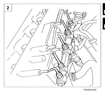
2. Undo the manifold side connectors for the pipes between the distribution manifold and the injectors and remove them.
