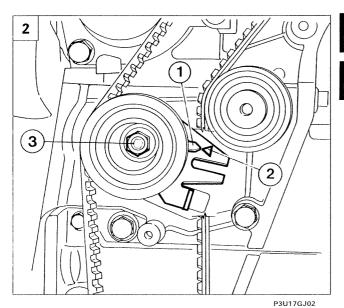
2 Loosen the nut fixing the tensioner (3) and, using a screwdriver for leverage in order not to completely discharge the tensioner, ensure that the moving reference (1) on the tensioner coincides with the fixed reference (2), then tighten the tensioner (3) fixing nut to a torque of 2.5 daNm.
