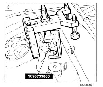
3. Undo the fixing nuts and carefully remove the injector bracket.
