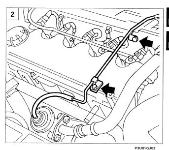
2. Undo the two bolts shown in the diagram and move the rigid pipe between the E.G.R. valve and the solenoid valve aside.
