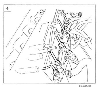
4. Undo the manifold side connectors for the pipes between the distribution manifold and the injectors and remove them.
