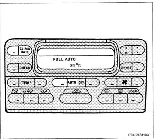
The controls which allow the use of the automatic climate control system are located in the INFOCENTER system which is in the centre of the dashboard.
