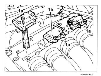
RIGHT CYLINDER HEAD IGNITION COILS
