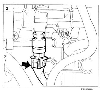
2. Disconnect the electrical connection from the fuel pressure sensor.
