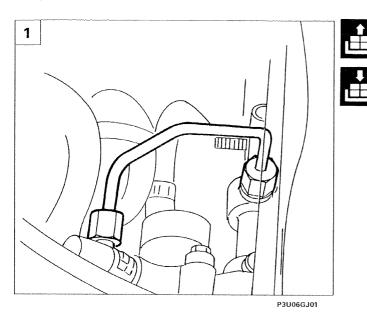
1. Remove the fuel supply pipe between the pressure pump and the distribution manifold.
