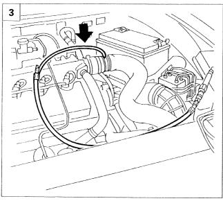
3. Connect the pressure transducer to tool 1870737000
