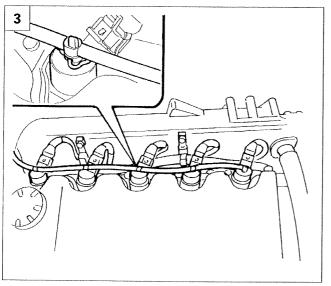
3. Disconnect the fuel return pipe from the injectors working on the spring.
