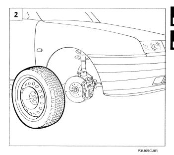
2. Position the vehicle on a lift and remove the right front wheel.
