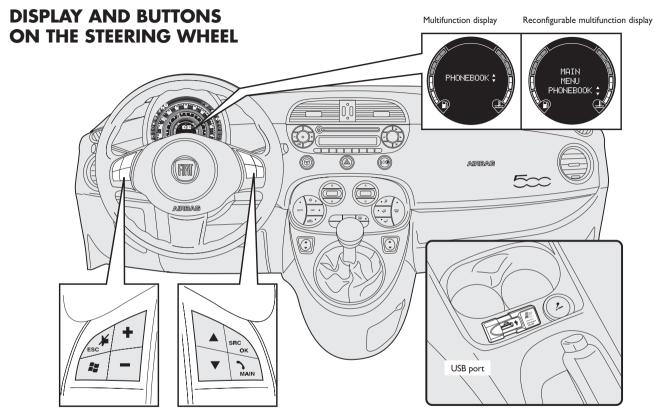
In this manual, the descriptions of the menu entries refer to the multifunctional display, which visualises some entries in abbreviated form compared to the version with reconfigurable multifunctional display. The reconfigurable multifunctional display visualises the menu entries in full.
