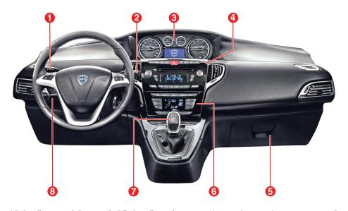
$1\ Left\ stalk:\ exterior\ lights\ control\ -\ 2\ Right\ stalk:\ windscreen\ wiper/rear\ window\ wiper/trip\ computer\ control\ 3\ Instrument\ panel\ -\ 4\ Radio\ (for\ versions/markets\ where\ provided)\ -\ 5\ Glove\ compartment\ 6\ Heating\ /\ Ventilation\ /\ Climate\ controls\ -\ 7\ Gear\ lever\ -\ 8\ Cruise\ Control\ stalk\ (for\ versions/markets\ where\ provided)$
