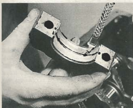
34.21 ... then lubricate the bearing shells
