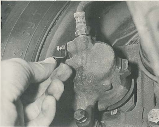
3.5 Pulling the dust cap from a front disc caliper bleed screw
