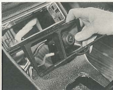
33.7 Removing the ashtray/cigarette lighter housing from the centre console
