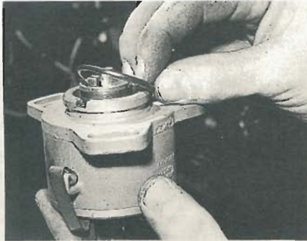
8.23 Examine the O-ring at the base of the distributor – 1.6 litre model
