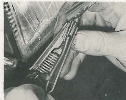
46.6B Disconnecting the washer fluid hose from the headlamp wiper arm
