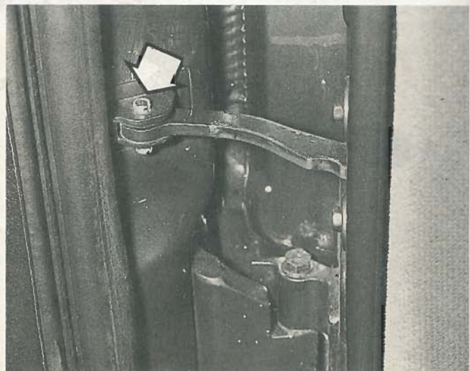
13.5 Front door check arm pivot pin (arrowed)
