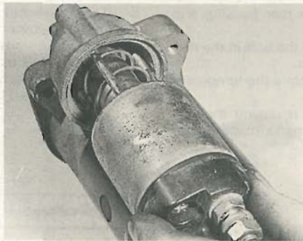
14.3A Withdraw the solenoid yoke ...
