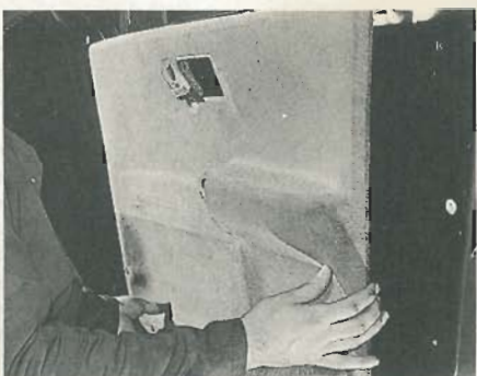
14.8 Removing a front door inner trim panel
