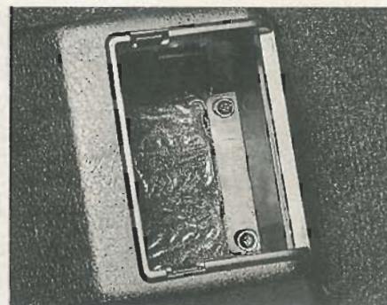
33.9 Centre console rear securing screws
