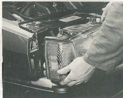
38.4C Withdrawing a headlamp assembly
