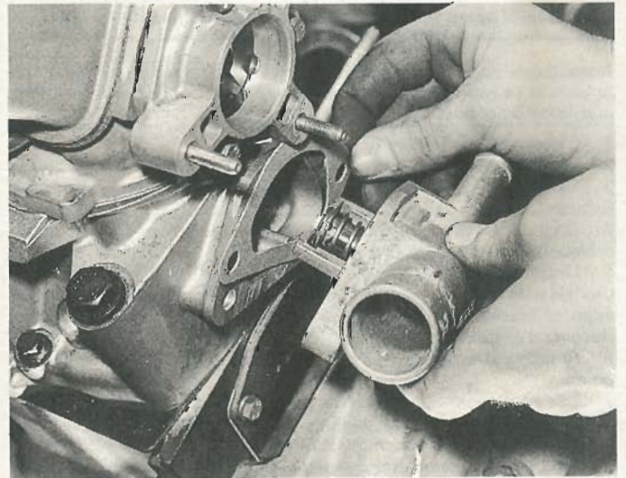
9.4B Removing the thermostat/cover assembly and the gasket (1.6 litre engine shown with distributor removed)
