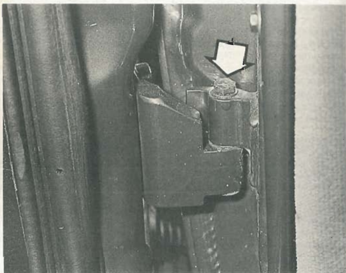
13.4 Front door hinge securing bolt (arrowed)
