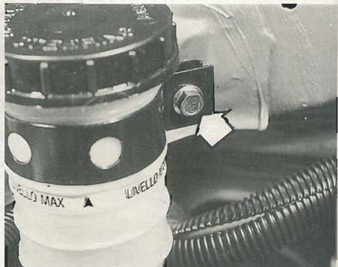
30.3 Power steering pump fluid reservoir clamp screw (arrowed)
