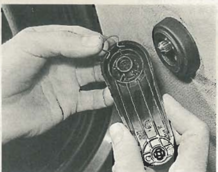
14.14C Rear door window regulator handle removed showing securing clip
