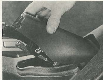
33.3 Withdrawing the cover from the handbrake lever
