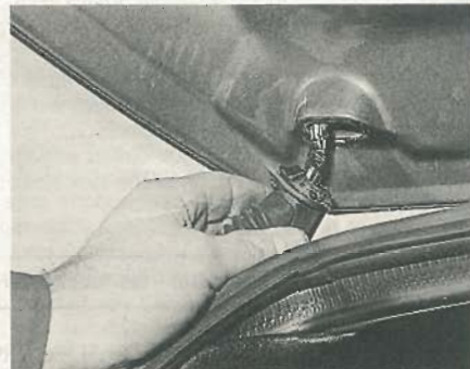
9.11 Pulling the wiring harness cover/tailgate buffer from the tailgate
