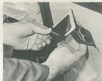
14.14D Removing a rear door interior handle trim
