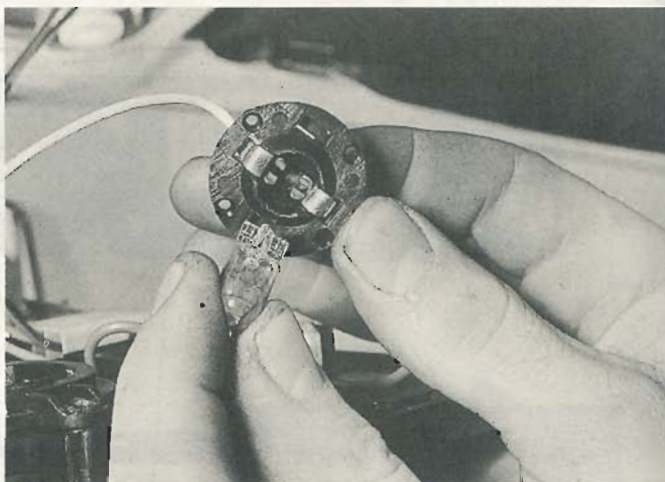
37.10 Renewing a map reading lamp bulb – model with sunroof
