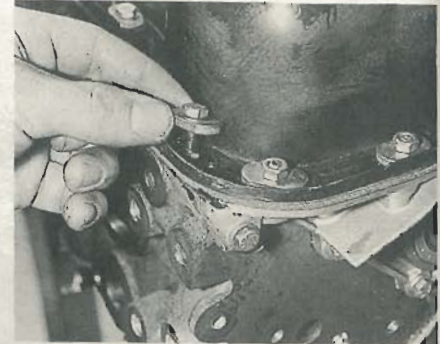
29.10C Refitting a sump securing bolt and washer plate
