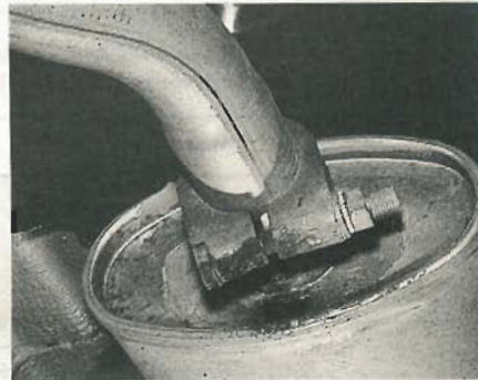
29.20 Exhaust centre-to-rear section clamp
