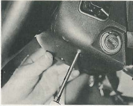
32.6 Extracting a lower steering column shroud securing screw
