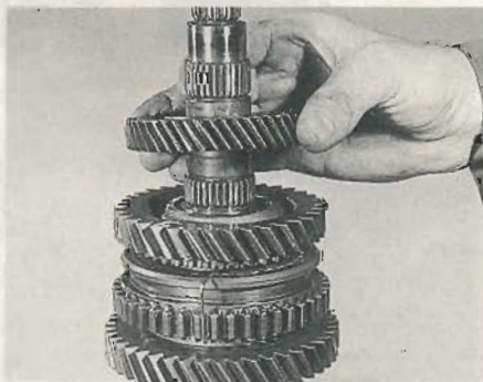
9.21 Fit the 3rd driven gear ...
