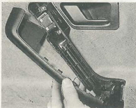
14.1 Removing a front door arm rest trim panel
