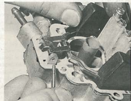
19.12 Removing the float pivot pin
