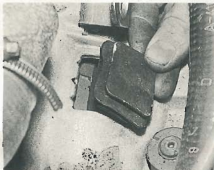
10.3 Removing the rubber cover from the timing aperture in the clutch bellhousing
