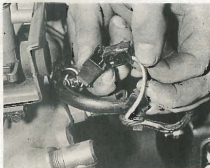
28.15 Disconnecting the inlet manifold heater wiring connector
