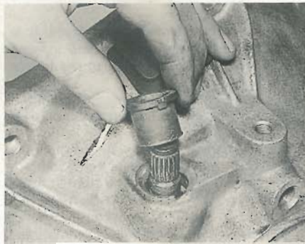
9.8A Remove the release fork rod upper bush ...
