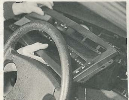
30.4B ... and lift the instrument panel from the fascia
