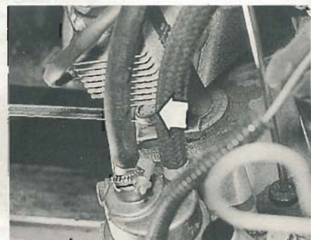
10.6 Loosening the distributor clamp bolt – 1.4 litre model
