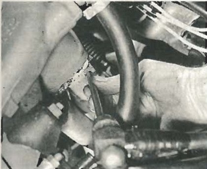
29.16C Using a drift to bend over a downpipe-to-manifold nut locktab
