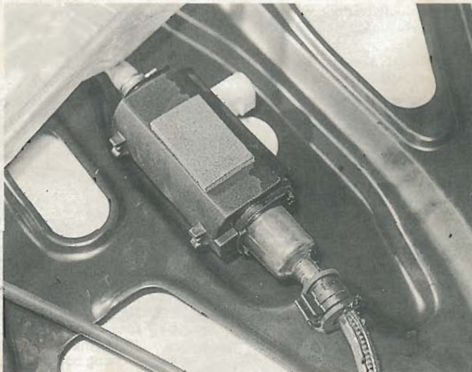
21.2 Front door electric window motor clipped to subframe
