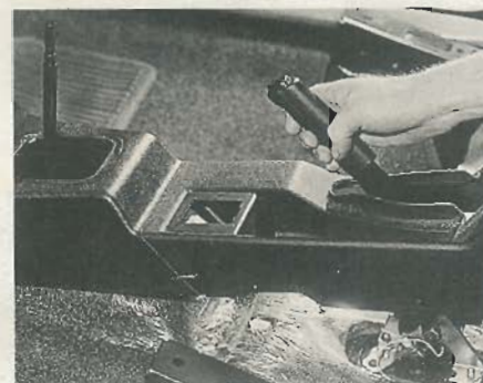
33.13 Removing the centre console
