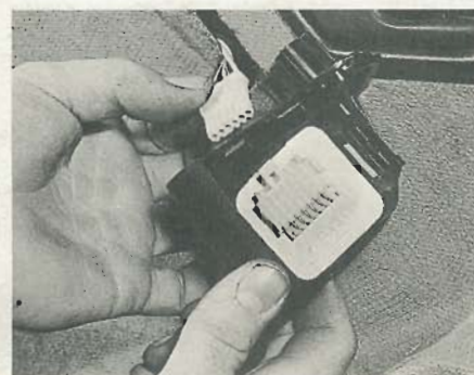
14.2B Disconnecting the electric windows switch wiring plug
