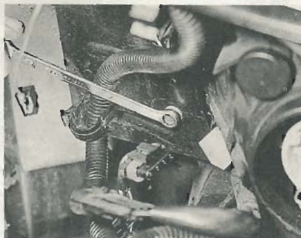
38.4B Unscrewing a headlamp securing bolt
