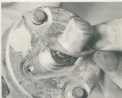
14.4 Removing the commutator end housing cap
