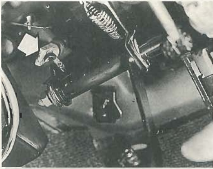
4.4 Unhook the end of the clutch cable (arrowed) from the pedal
