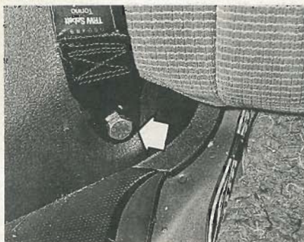
36.9 Rear seat belt lower mounting (arrowed)
