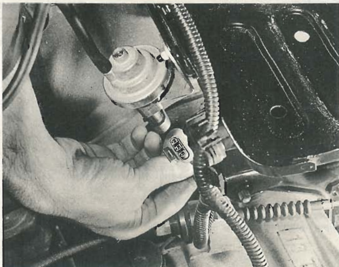
61.3 Disconnecting the wiring plug from the economy gauge sender unit
