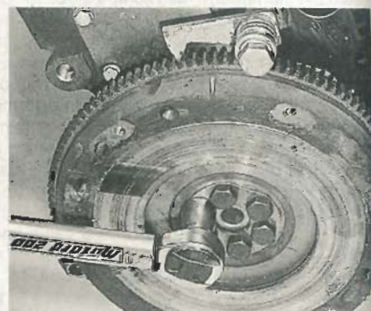
26.9B ... and tighten the bolts to the specified torque. Note tool used to prevent flywheel turning
