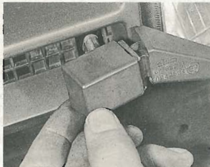
46.6A Removing the cover from the headlamp wiper arm securing nut
