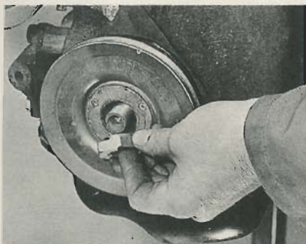
15.3A Removing the crankshaft pulley nut ...
