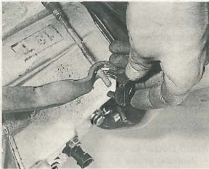
4.11 Withdraw the plastic block from the release arm
