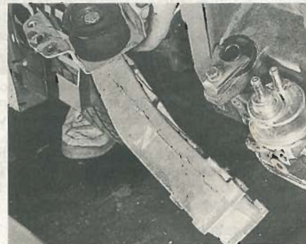
9.25 Withdrawing the right-hand engine mounting assembly
