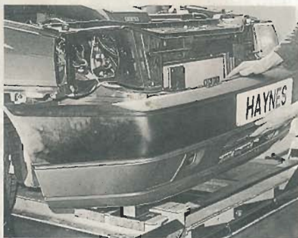
23.5 Withdrawing the front bumper
