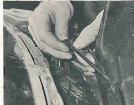
25.5B ... and disconnect the washer fluid hose connector
