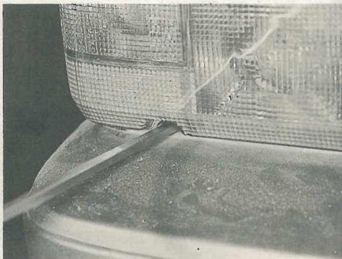
42.3A Extracting a rear lamp unit securing screw
