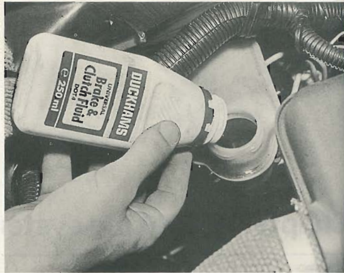
2.2 Topping-up the brake fluid level
