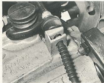
4.12 Cable sheath rubber grommet (arrowed) on gearbox casing
