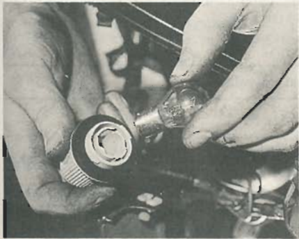
44.9 The front direction indicator lamp bulb is a push-fit in the bulbholder
