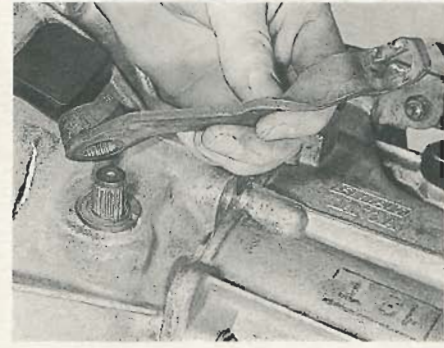
9.7B ... and remove the clutch release arm
