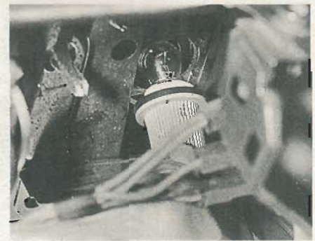
44.8 Removing a front direction indicator lamp bulbholder
