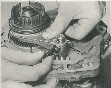
7.8 Extract the securing screw and move the 5th gear selector fork downwards to engage 5th gear
