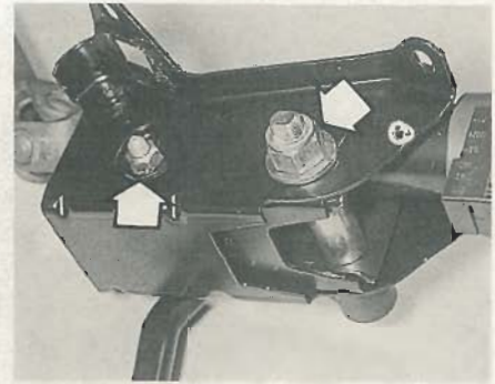
21.15 Steering column tube-to-mounting bracket nuts (arrowed) – adjustable steering column
