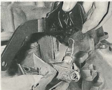
13.25A Refit the external lever assembly ...
