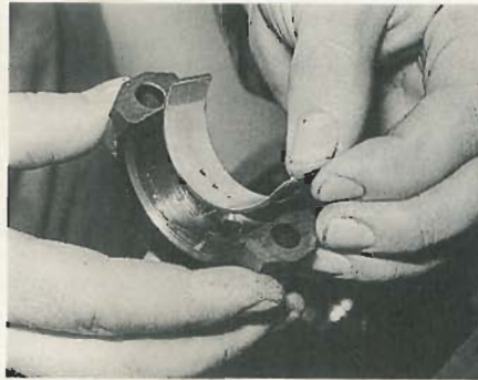
32.12 Fitting the bearing shell to a big-end bearing cap
