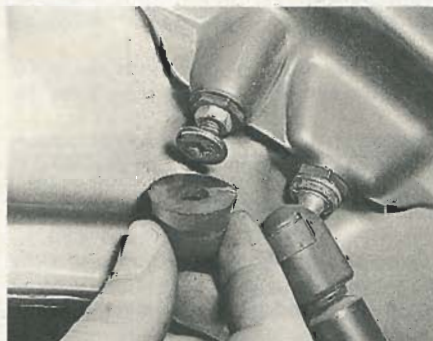
9.19 Tailgate buffer rubber removed to expose buffer pin
