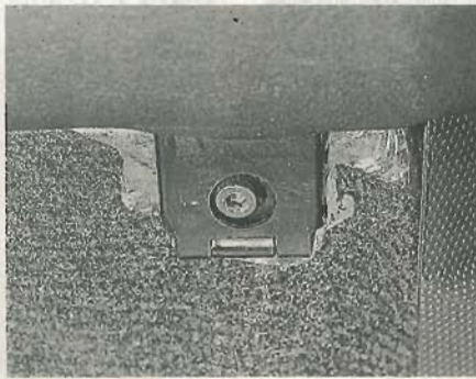
35.6 Rear seat cushion hinge securing bolt
