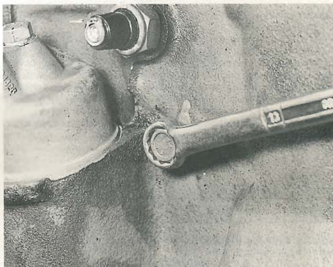
3.5 Unscrewing the cylinder block drain plug
