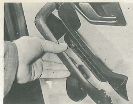
14.14A Removing the rear door arm rest trim panel
