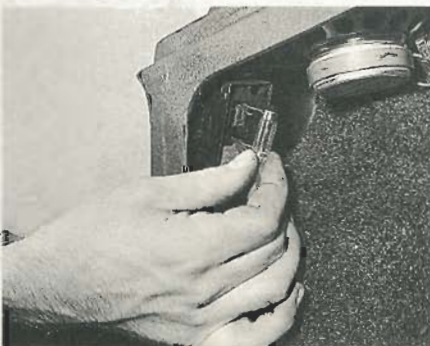
37.14 Removing the luggage compartment lamp bulb
