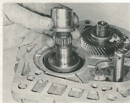
15.26B ... and the sleeve to the input shaft
