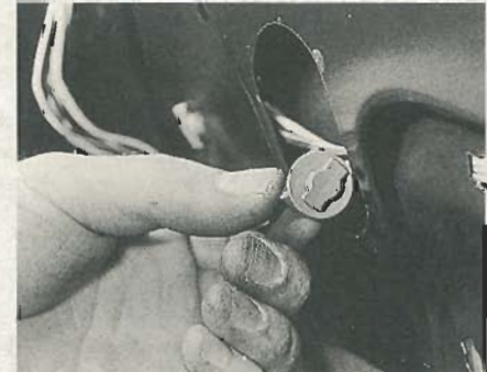
15.6B ... to release the wiring harness from the front door subframe
