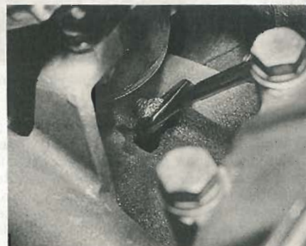
28.20A Unscrewing an exhaust manifold securing nut
