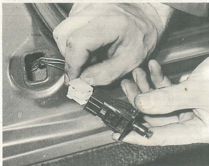
22.4 Disconnecting the wiring plug from a door-operated courtesy lamp switch
