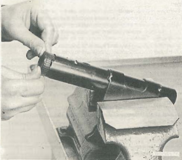
Fig. 9.7 Renewing a steering column bush (Sec 21)
