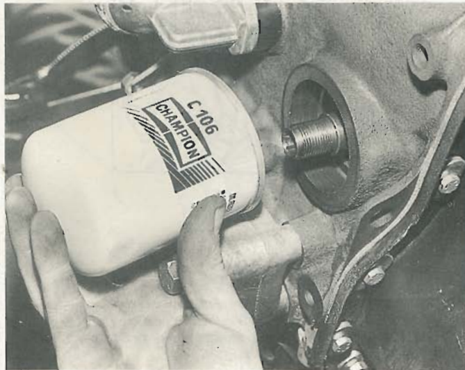
3.7 Fitting a new oil filter
