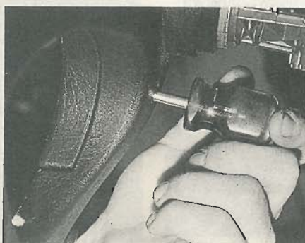
20.3B Removing a horn-push pad securing screw – DGT model
