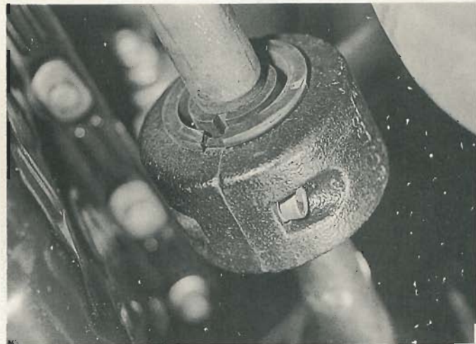
9.1 Right-hand driveshaft damper weight
