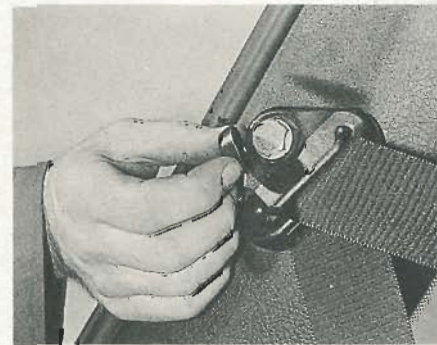
36.10 Removing the trim to expose the rear seat belt upper mounting bolt
