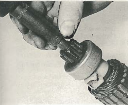
14.12A Drive the collar down the shaft ...
