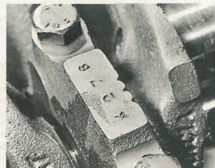
34.7 Identification notches on No 3 main bearing cap
