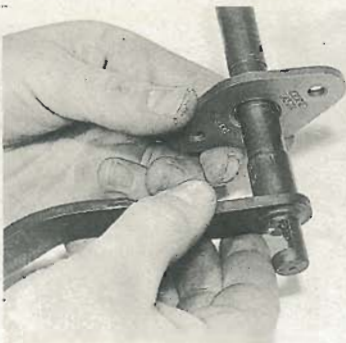
13.14 Sliding the mounting plate over the gear selector shaft
