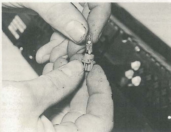
31.23B ... the bulb is a push-fit in the bulbholder - digital instrument panel
