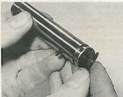
15.4 Fitting a new reverse idler shaft O-ring
