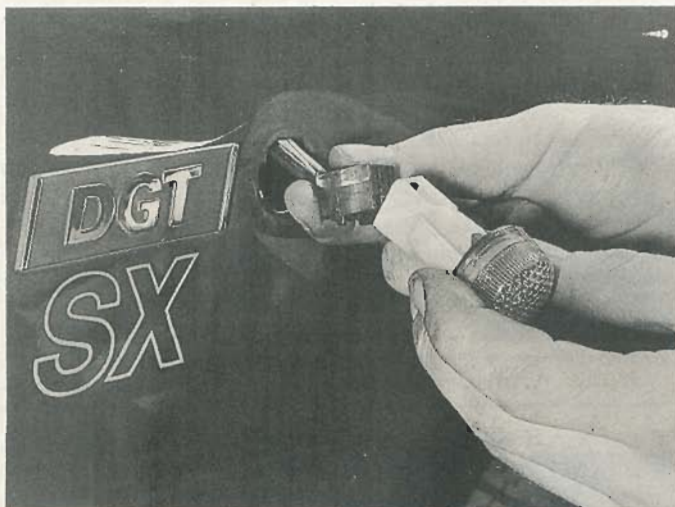
41.4 Removing a front direction indicator side repeater lamp assembly
