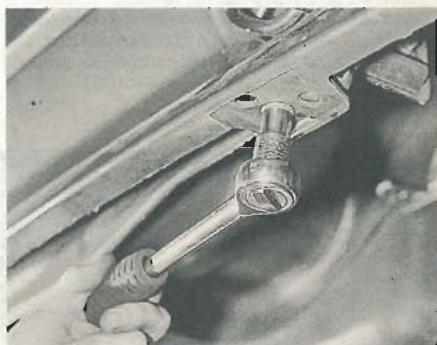
23.11 Unscrewing a rear bumper lower securing bolt
