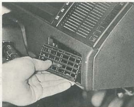
32.26 Removing a fascia ventilation nozzle
