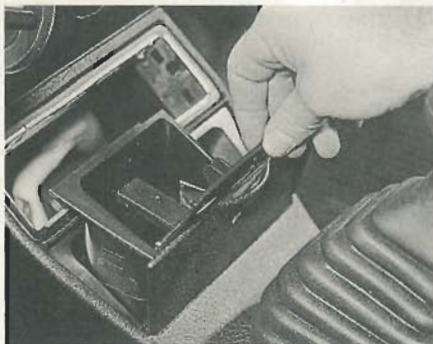
33.6 Removing the front ashtray from the centre console
