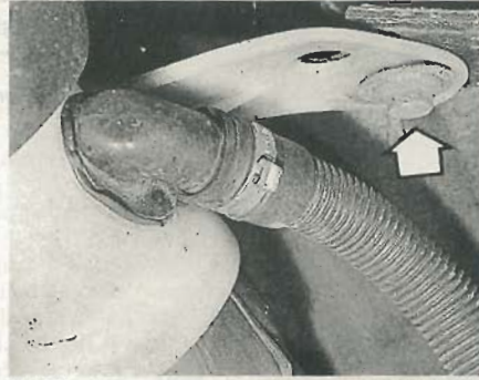
10.7 Fuel filler tube securing screw (arrowed)
