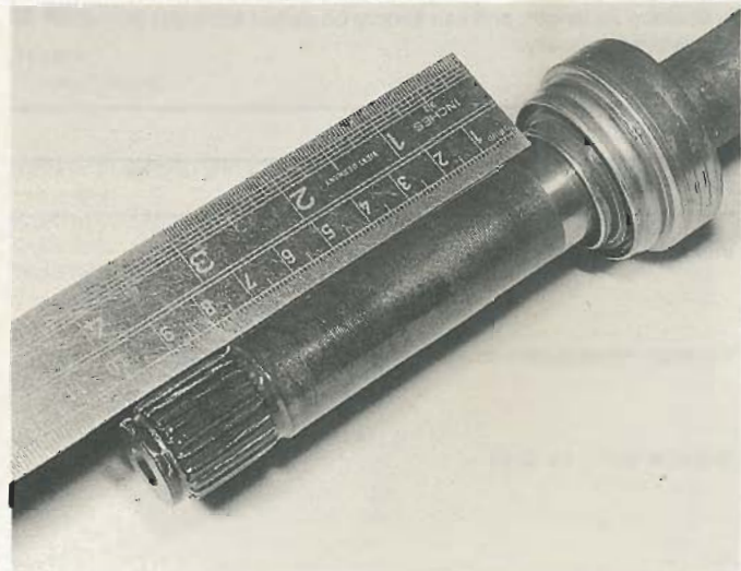
8.4 Measure the exact distance of the bearing from the inboard end of the driveshaft
