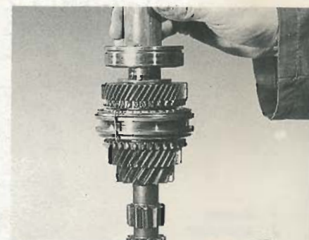
8.17 Drive the bearing down the shaft using a piece of tubing
