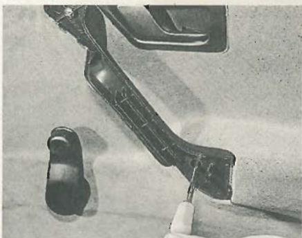
14.14B Extracting a rear door arm rest securing screw
