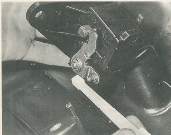
11.4B Disconnecting the lock operating rod from the tailgate lock cylinder assembly
