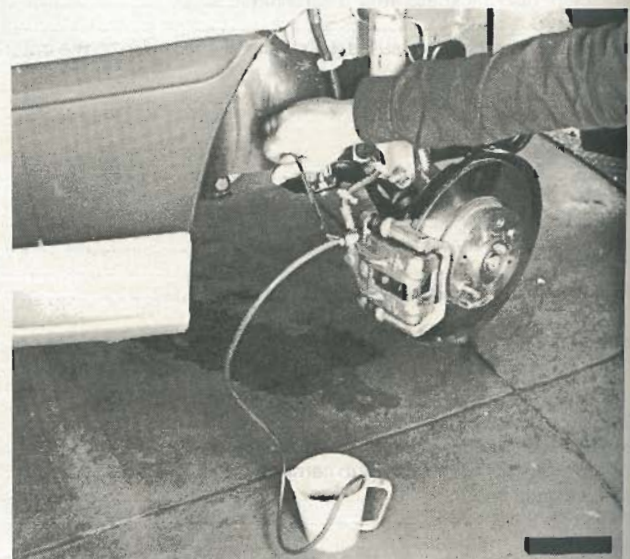
Fig. 8.1 Bleeding a front brake (Sec 3)
