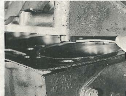
21.17B ... so that the positioning dowels engage in their holes
