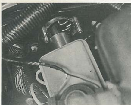
15.4 Withdraw the brake master cylinder from the studs on the servo
