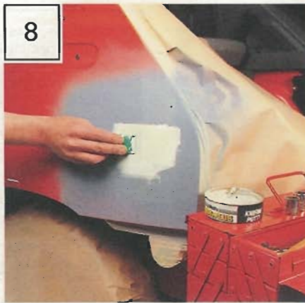
8 Fill any imperfections in the filler surface with a small amount of Holts Body Plus Knifing Putty. Using plenty of clean water, rub down the surface with a fine grade wet-and-dry paper - 400 grade is recommended - until it is really smooth.
