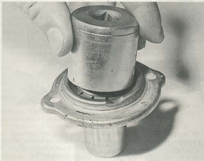
12.5 A suitable socket can be used to drive the input shaft oil seal into the guide sleeve
