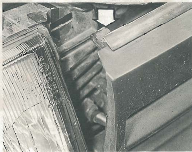
24.4 Withdrawing the grille panel – securing clip arrowed
