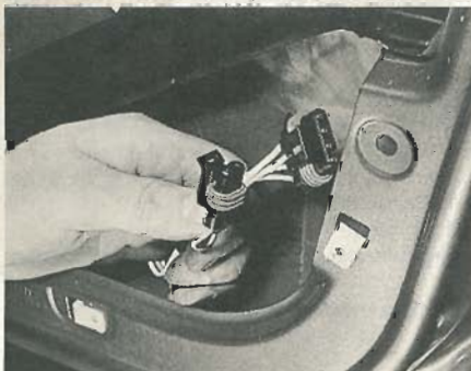
15.5 Disconnecting the wiring plugs from the front door central locking motor
