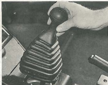
33.4 Removing the gearchange lever knob/gaiter moulding
