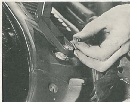
46.2 Removing a windscreen wiper arm securing nut
