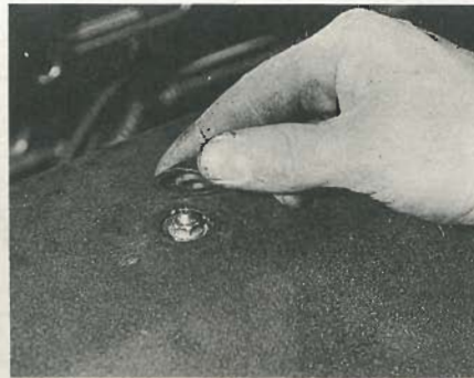
5.3A Remove the rubber cover from the air cleaner securing nut ...
