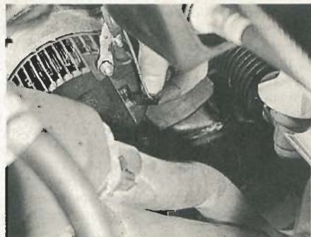
8.2 Disconnecting the alternator wiring plug
