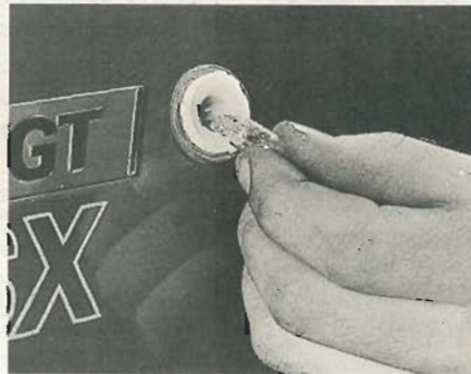
44.12 Removing a front direction indicator side repeater lamp bulb
