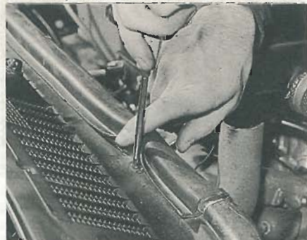
25.4 Extracting a windscreen cowl panel lower securing screw
