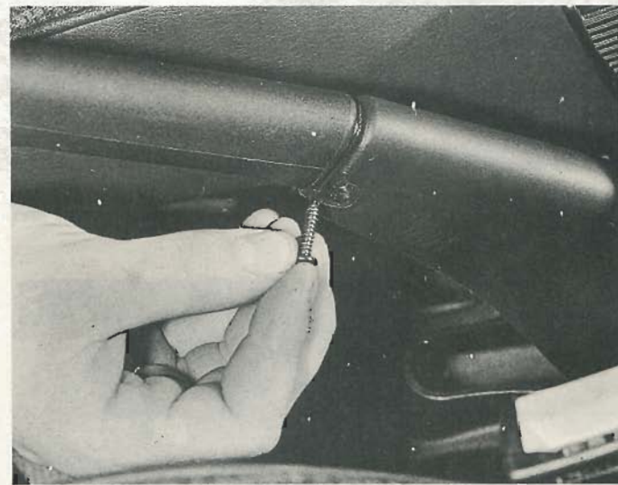
17.3 Removing the handbrake lever cover securing screw
