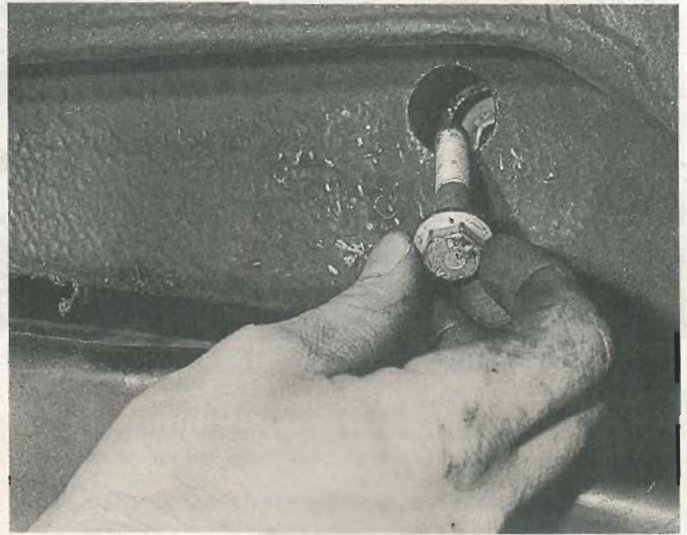
15.4 Removing a rear shock absorber upper mounting bolt
