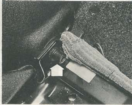
35.9 Outer seat back hinge-to-body bolt (arrowed)
