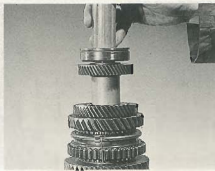
9.24 Drive the bearing down the shaft using a piece of tubing
