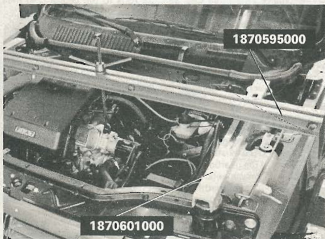
Fig. 6.3 FIAT special tools used to support engine during gearbox removal (Sec 5)
