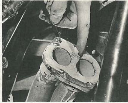
29.16A Coating the exhaust downpipe mating face with assembly paste
