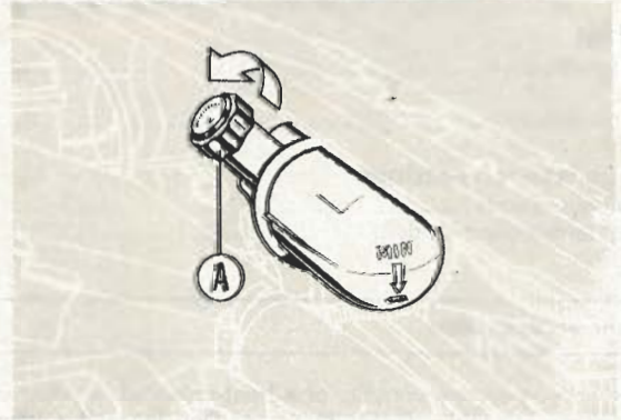
Fig. 2.2 Coolant expansion tank location and MIN level mark (Sec 2)
