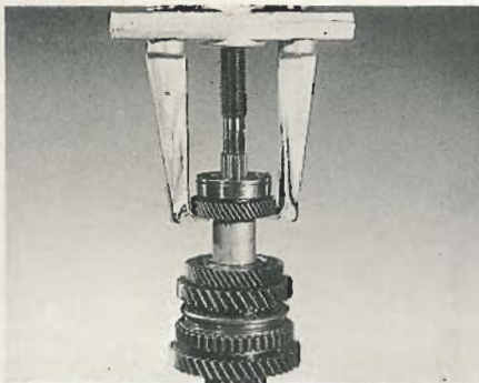
9.2 Using a puller to remove the bearing and 4th driven gear from the mainshaft
