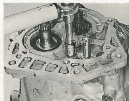
15.24B ... and tighten the securing bolt
