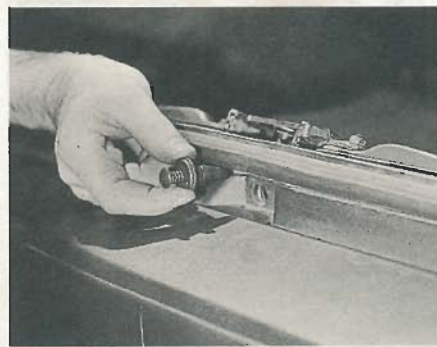
23.9 Withdrawing the expanding fastener and securing bolt from the rear bumper
