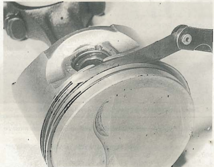
33.7B Measuring a piston ring-to-groove clearance
