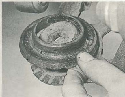
16.3 Removing a rear coil spring lower mounting rubber
