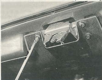
9.5 Removing a tailgate trim panel/lock securing screw
