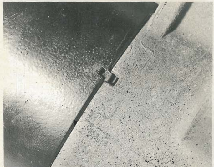
14.22 The lug on the yoke must engage with the cut-out in the drive end housing
