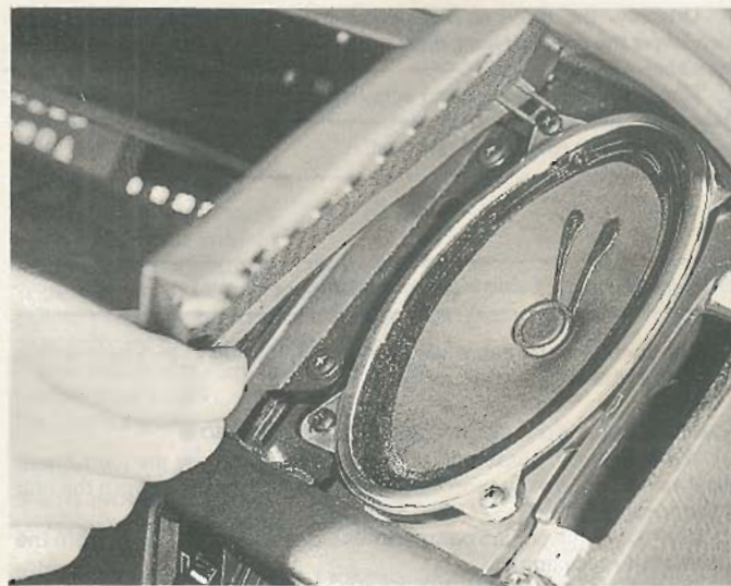
56.2 Removing the trim panel to expose the facia-mounted loudspeaker
