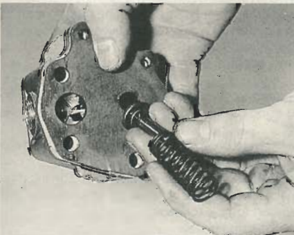
31.13A Locate the pressure relief valve and spring on the intermediate plate
