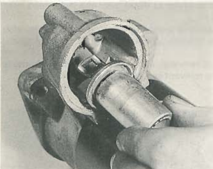
14.3C ... then unhook the armature from the actuating arm
