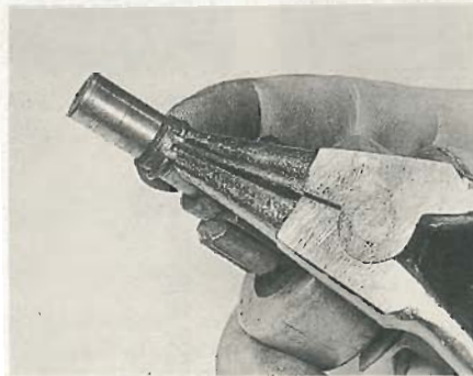
14.12B ... and remove the drive pinion retaining C-clip
