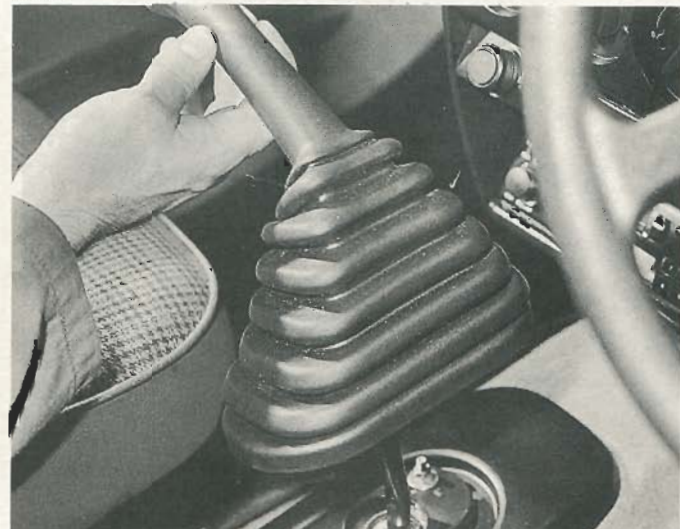
4.1 Removing the gearchange lever knob/gaiter moulding – model without centre console
