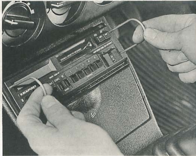
57.3 Using DIN tools to remove the radio/cassette player
