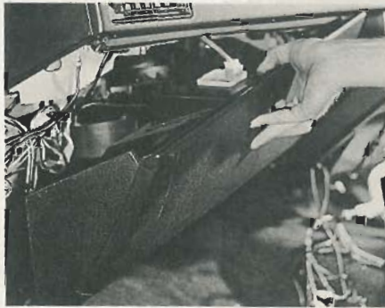
32.11A Withdraw the glovebox assembly ...
