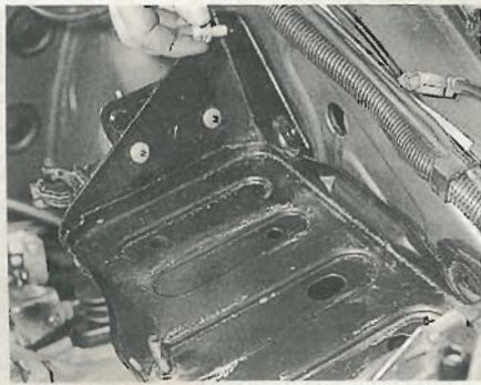
10.12 Removing an upper securing bolt from the battery tray
