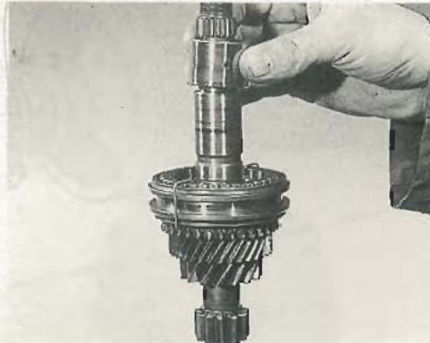
8.13 ... followed by the 4th gear bearing sleeve
