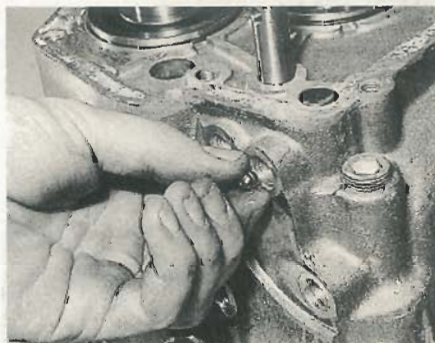
15.21A Refitting a detent ball, ...
