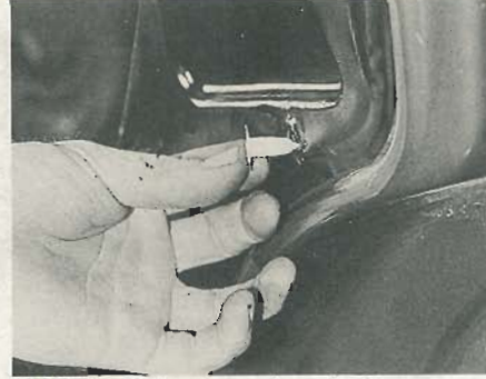
14.14F Removing a rear door plastic insulating sheet securing clip
