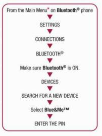
You can activate **Blue&Me<sup>TM</sup>** menu through steering wheel controls, by pressing button and vocally by pressing the hand-free button and speaking out the feature you would like to activate loudly. Follow the logic as it is shown below:
