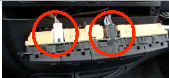
Now pull the switches out and disconnect the connectors circled red.
