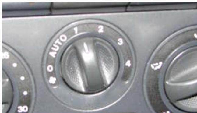
The next screw is hidden under the fan speed button. So pull it off and unscrew the screw pointed by an arrow.
