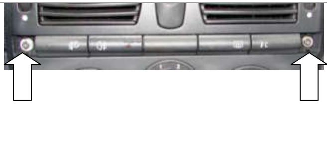
When that is done you will have 2 screws visible like on the pic. Unscrew the screws pointed with arrows.
