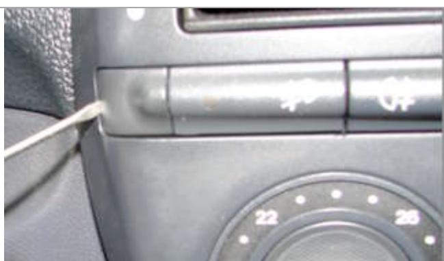
Then using a screwdriver or a knife prize out the ends of the switch line.
